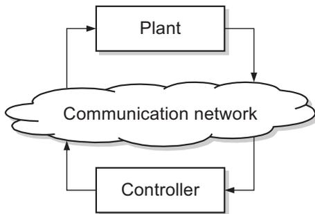
Figure 1: Basic structure of a networked control system
