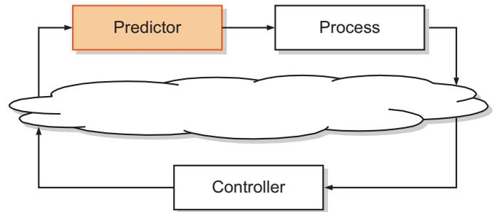
Figure 5: Structure of a predicted networked control system
