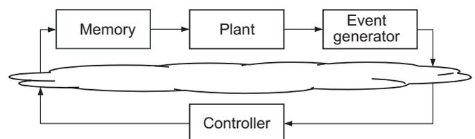
Figure 3: Structure of an event-driven control system
