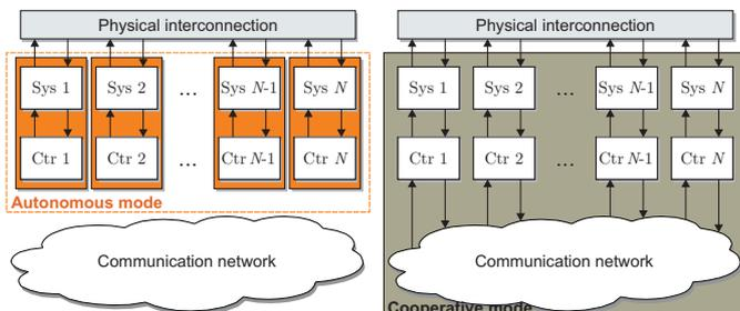
Figure 1: Control of interconnected systems in autonomous mode and cooperative mode
