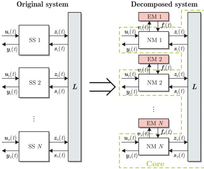
Figure 2: Decomposition of similar subsystems in a core of identical subsystems and error models
