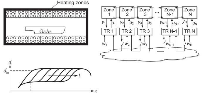
Figure 3: Multizone crystal growth furnace
