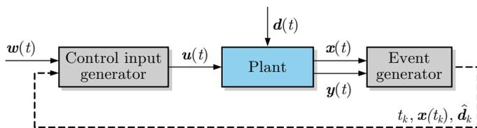
Fig. 1: Event-based control loop
