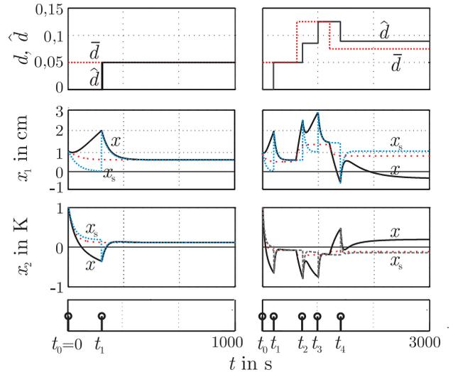
Fig. 4: Behaviour of the process model subject to two different exogenous disturbances
