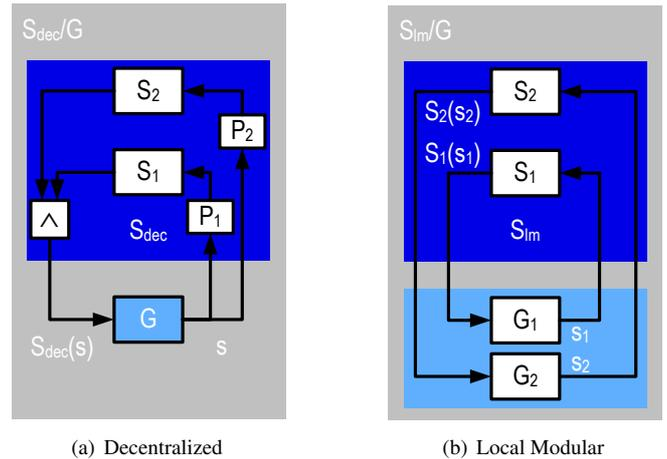
Figure 4: Structured supervisory control synthesis
