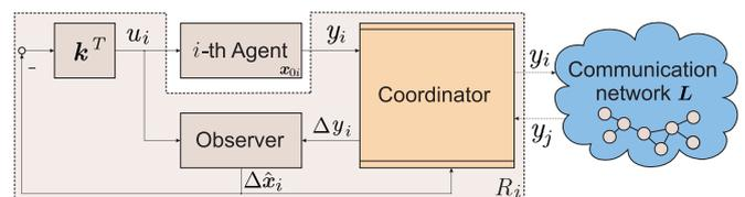
Figure 2: Structure of the control algorithm
