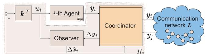
Figure 2: Structure of the control algorithm
