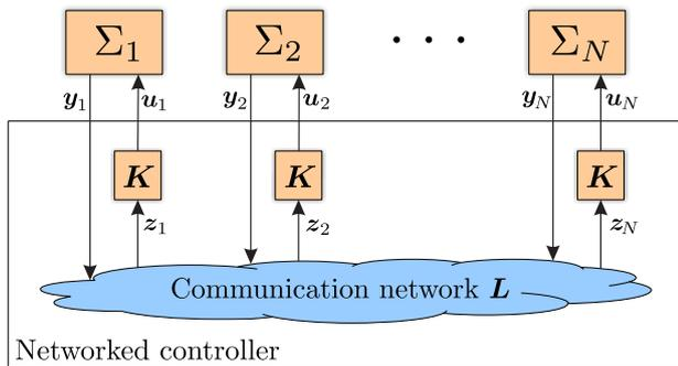
Figure 1: Multi-agent system linked to a uniformly weighted communication topology by networked controller
