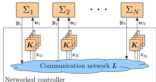
Figure 2: Multi-agent system linked to an arbitrary weighted communication topology by networked controller
