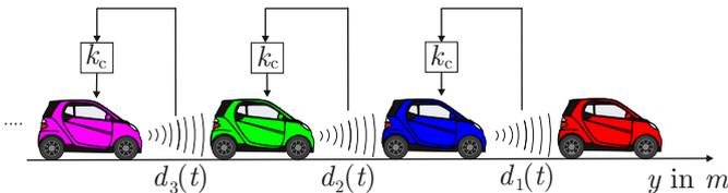
Figure 1: Platoon of cars with radar sensors
