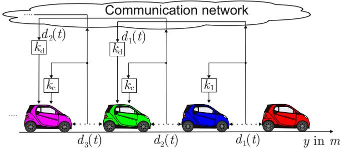
Figure 2: Platoon with communication network
