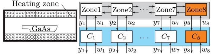
Figure 3: Multizone furnace for crystal growth
