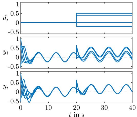
Figure 3: Step disturbances (top), oscillator network without local controller and oscillator network with networked controller which satisfies the internal-model principle.
