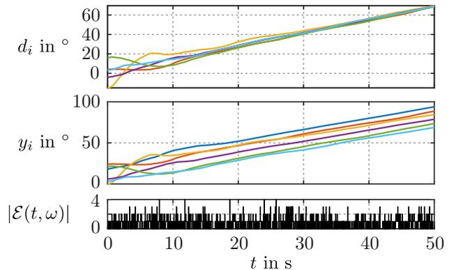
Figure 4: Distances (top) and position (middle) of the mobile robots and the number of active communication links over time (bottom)
