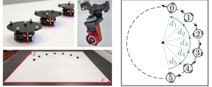
Figure 3: Experimental set-up SAMS (left) and synchronisation of the distances between mobile robots (right)
